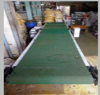
5 Meter Truck Loading Conveyor
