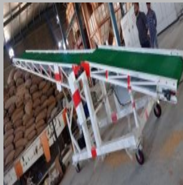
9 Meter Truck Loading Conveyor
