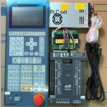
Programmable Logic Controller System
