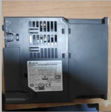
Delta VFD AC Drive
