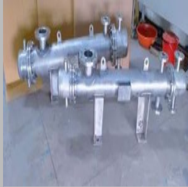
Chiller Heat Exchanger
