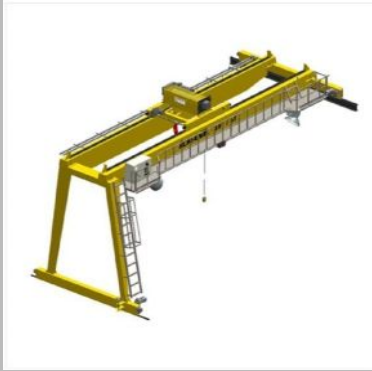
Semi Gantry EOT Crane
