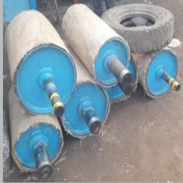
Mild Steel Belt Conveyor Head Pulley
