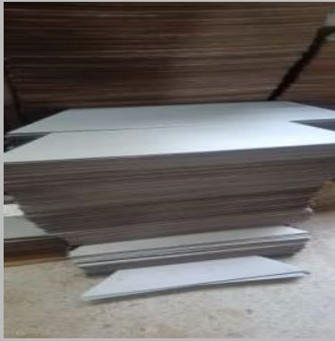
100 KVA Transformer Lamination
