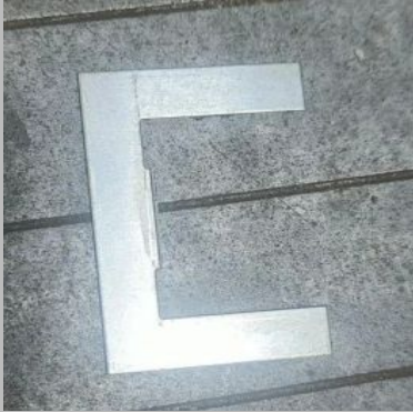
U Transformer Lamination
