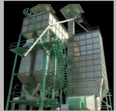
Paddy Dryer Heat Exchanger
