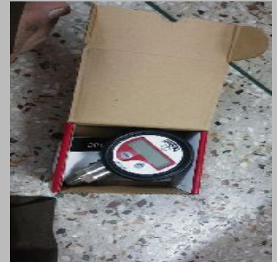
Winters Digital Pressure Gauge Model No DPG222R11
