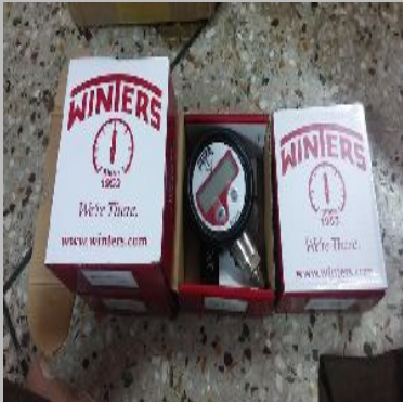
Winters Digital Pressure Gauge Model No DPG205R11
