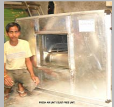
Fresh Air Unit, Dust Free Unit
