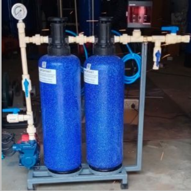
Industrial DM Water Plant
