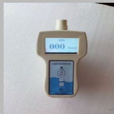
Industrial Hydrogen Gas Leak Detector
