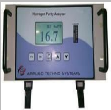
Turbine Process Gas Anlazer
